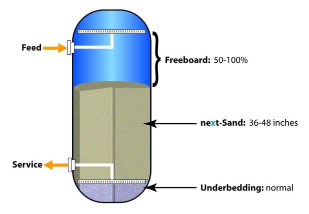
Sizing guidline: 12-20 gpm /ft2 depending on filtrate quality target and contaminant load.
