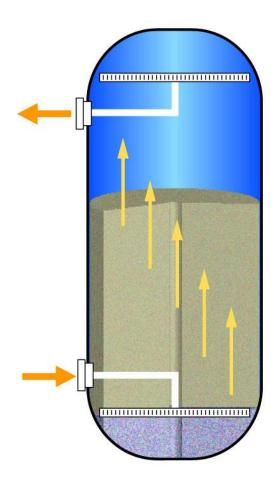
Backwash at 15 to 17 gpm/ft<sup>2</sup> for 10 to 15 minutes.
